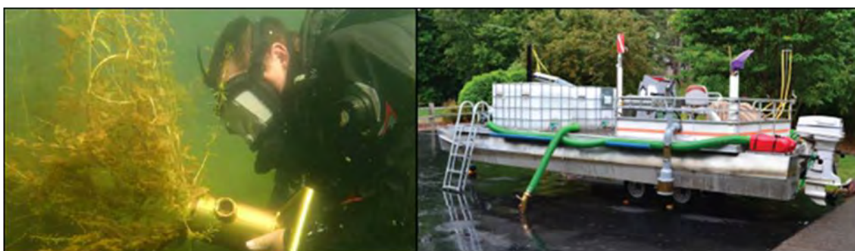
Figure 47: DASH – Feeding EWM into the underwater Suction Hose (Marinette Co.); and a sample DASH Pontoon Boat (Beaver Dam Lake Management District)
