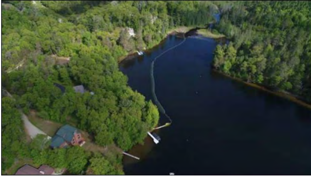
Figure 53: Limno-curtain installed on Thunder Lake (photo from Marinette Co. LWCD)
